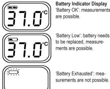
**Battery Indicator Display** 'Battery OK': measurements are possible.
